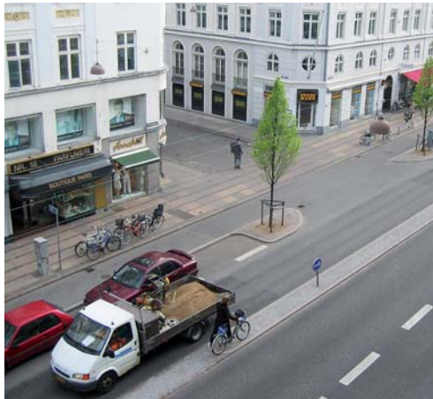
Image 30 Junction demarcation with street trees. Note the continuous footway across the junction; Copenhagen
