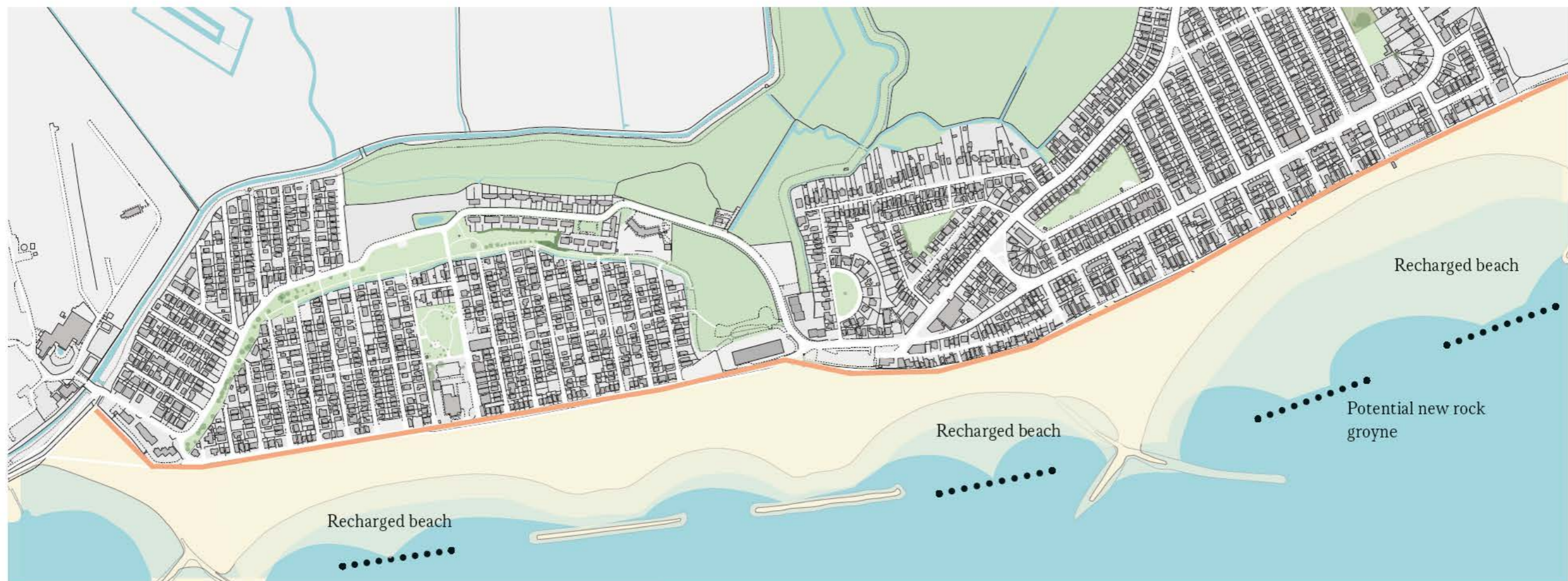
Fig. C39. Map indicatively showing Option C, with reshaped beach and potential locations of new rock groynes (dotted)
