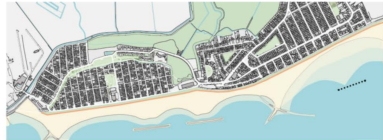
Fig. C41. Map showing line of new sea of wall proposed under Option B, and location of potential additional rock groyne
