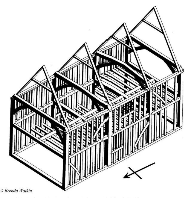
Figure 27: Spring Road, the timber frame of no. 8, the former guildhall (Brenda Watkin)
