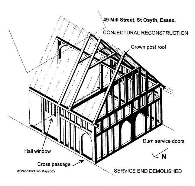
Figure 38: The timber frame of 49 Mill Street, a 15th-century hall with the cross-passage door and the pair of doors to the now demolished service end (Brenda Watkin).
