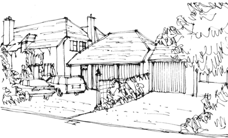
12. The design of these garages and their open forecourts not only disrupt the mature planting along Church Lane but also affect the setting of Wood Hall, one of the Area's most significant and attractive houses. The sketch shows potential solutions for the garages in keeping with the character of this distinctive building.
